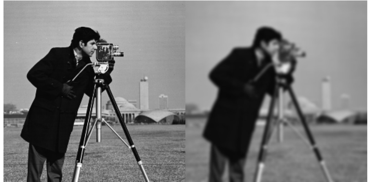
Original Image (Left) Vs. Gaussian Filtered Image (Right)
